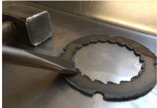
Fig 2. Image of slag on the back of the cut steel.
