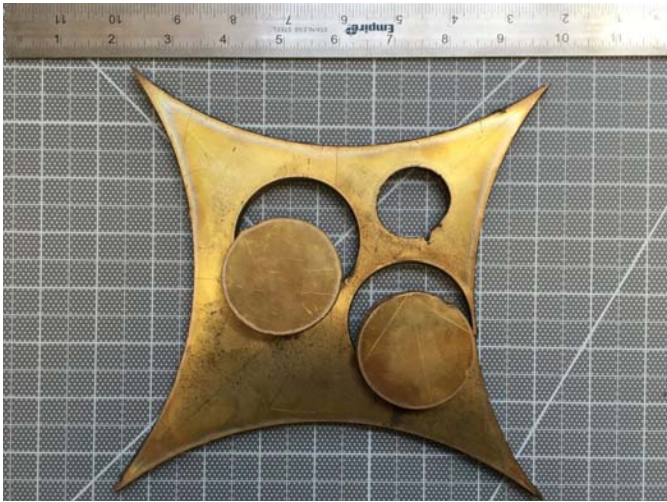
Fig 3. Brass (1/2" thick) cut with plasma cutter.
