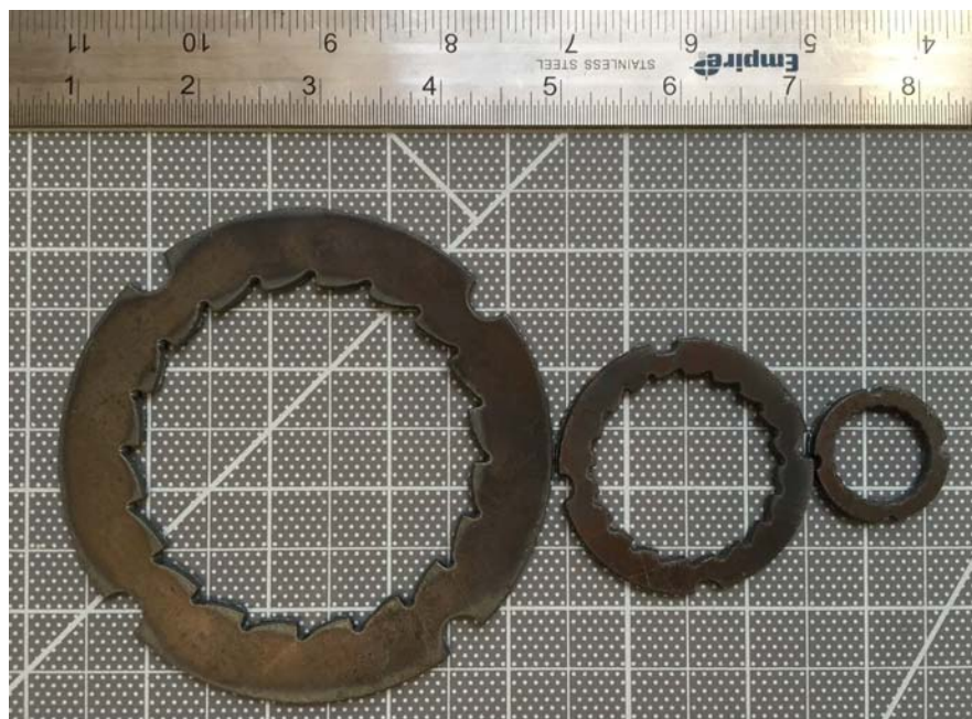
Fig 5. Shows loss of detail in the cut as the object becomes smaller.
